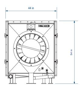
Fan Motor: 3 phase, 72 hp, 480/520V, 60 Hz
