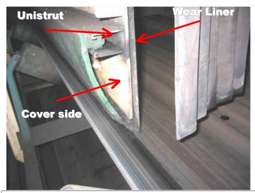
Installation with Snap-In and single Unistrut piece. Mounting at 14" from bottom of wear liner. Caulking on top of Unistrut to stop dust leaks.
