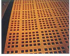
Unlike standard tension mats, the RhinoGrid extends all the way to the hooks, thereby increasing the open area.
